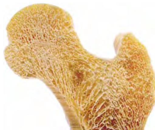
Figure 3. A noncalcined cancellous bone (femoral head) showing the transition from a more compact outer layer ( corticalis ) to a more porous interior ( spongiosa ).
