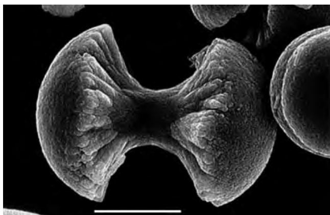
Figure 13. A biomimetically grown aggregate of fluoroapatite that was crystallized in a gelatin matrix. The crystal shape can be explained and simulated by a fractal growth mechanism. Scale bar: 10 \mu\text{m} (taken from ref. [252] with permission).
