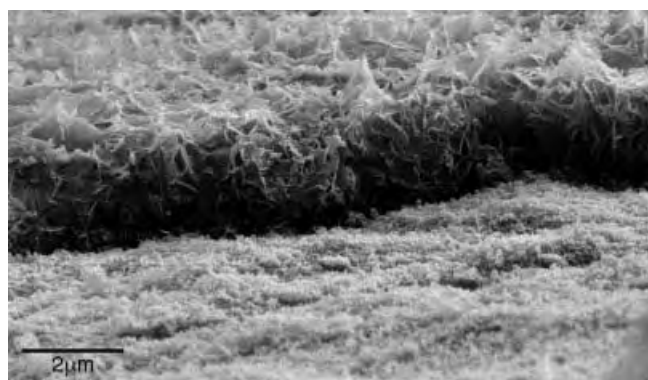
Figure 12. The surface of a nickel–titanium shape-memory alloy (“Nitinol”) that was coated with a calcium phosphate layer by dipping into an supersaturated calcium phosphate solution. The front part shows the etched metal surface from which the calcium phosphate layer has been mechanically removed. Scale bar: 2 \mu\text{m} .
