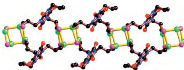
Figure 1. The chain structure of 1 which extends in the c direction (Cu green, Br pink, O red, N blue, C black). The open-cubane unit is highlighted with yellow bonds. H atoms have been omitted for clarity. Typical bond lengths [Å]: Cu–Br 2.422–2.395, Cu–C 2.063–2.106, coordinated olefin C=C 1.347–1.402.
